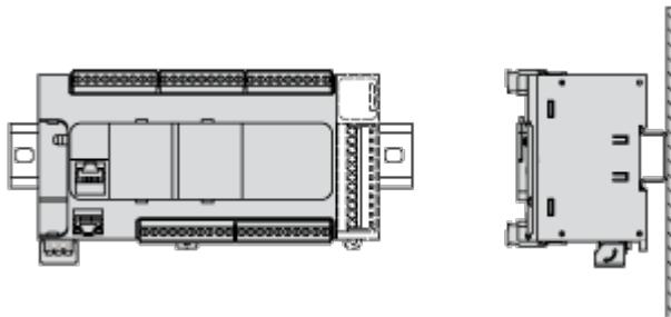
**Acceptable Mounting Position**
