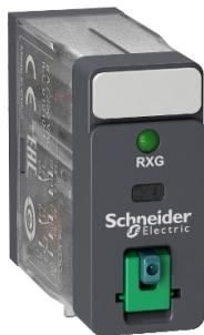
interface plug in relay, Harmony Electromechanical Relays, 5A, 2CO, with LED, lockable test button, 48V DC
