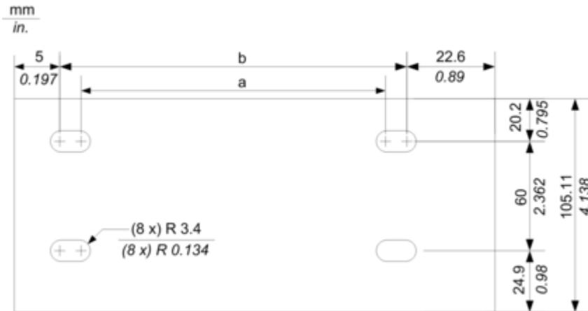
**NOTE:** You can use M4, M5, M6, or UNC #6 screws in the fastening holes.
