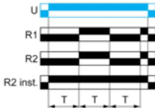
**Function: 1 Output with Retrigger / Restart Control**
