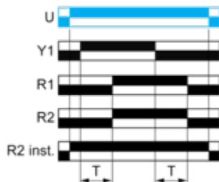
**Function At : Power on Delay Relay (Summation) with Control Signal**
