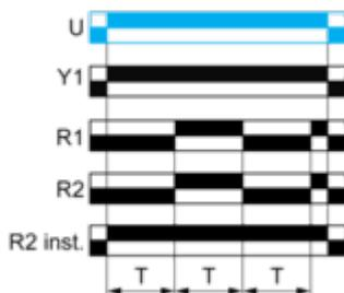
Function Di : Symmetrical Flasher Relay (Starting Pulse On)**Description**
