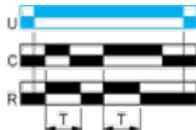
**Function Bw : Double Interval Relay with Control Signal**
