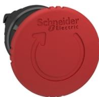
Emergency stop head, Harmony XB4, switching off, black metal, red mushroom 40mm, 22mm, trigger latching turn to release
