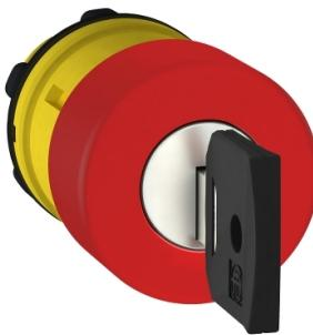
Emergency stop head, Harmony XB5, switching off, plastic, red mushroom 30mm, 22mm, trigger latching key release
