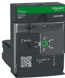
Standard control unit, TeSys Ultra, 3P, 1.25 to 5A, 690VAC, thermal magnetic protection, class 10, 24VAC coil
