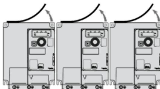
**Mounting Type C: Individual, Ventilation Cover Removed**
