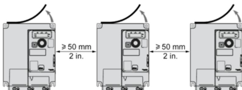
For Operation at Ambient Temperature Above 50 °C (122 °F)
