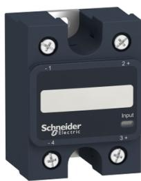
single phase relay, Harmony Solid State Relays, 50A, panel mount, zero voltage switching, thermal pad, input 4 to 32V DC, output 48 to 660V AC
