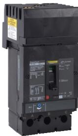
Circuit breaker, PowerPacT J, 250A, 3 pole, 600VAC, 100kA, I-Line, thermal magnetic, 80%, ABC
