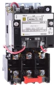
NEMA Motor Starter, Type S, nonreversing, Size 1P, 36A, 5 HP at 230 VAC, 5 kA SCCR, 1 phase, 2 pole, melting alloy, 240 VAC coil, open [TAA]
