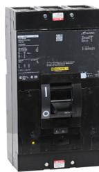
Circuit breaker, LH, 350A, 3 pole, 600VAC, 25kA, 250VDC, 50kA, lugs, thermal magnetic
