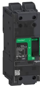
Circuit breaker, PowerPact B, 90A, 2 pole, 600Y/347VAC, 14kA, lugs, thermal magnetic, 80%
