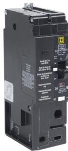
Mini circuit breaker, E-Frame, 30A, 1 pole, 277VAC, 25kA max, bolt on, 30mA ground fault protection [TAA]
