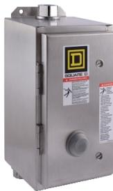
NEMA Motor Starter, Type S, nonreversing, Size 0, 18A, 5 HP at 460 VAC, 5 kA SCCR, 3 phase, 3 pole, melting alloy, 120 VAC coil, NEMA 4/4X [TAA]
