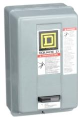
NEMA Motor Starter, Type S, nonreversing, Size 0, 18A, 5 HP at 460 VAC, up to 100 kA SCCR, 3 phase, 3 pole, Motor Logic, 240 VAC coil, NEMA 1 [TAA]
