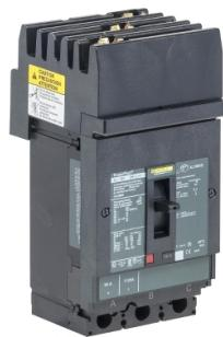
Circuit breaker, PowerPact H, 90A, 3 pole, 600VAC, 25kA, I-Line, thermal magnetic, 80%, padlock handle, ABC
