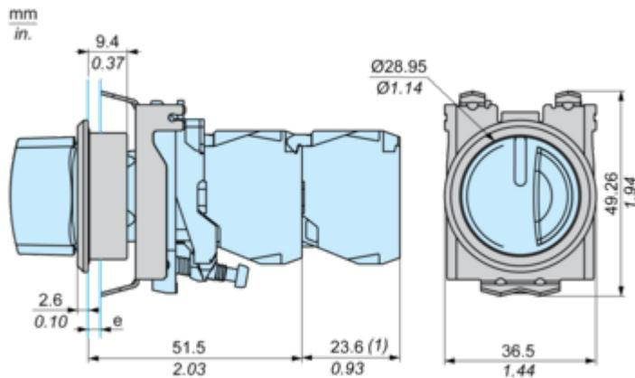
e : Clamping thickness : 1.2 to 2.8 mm / 0.05 to 0.11 in.
