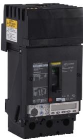
Circuit breaker, PowerPact J, 250A, 3 pole, 600VAC, 14kA, I-Line, Micrologic 5.2A, 80%, ABC
