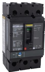
Circuit breaker, PowerPacT J, 250A, 3 pole, 600VAC, 25kA, lugs, thermal magnetic, 80%
