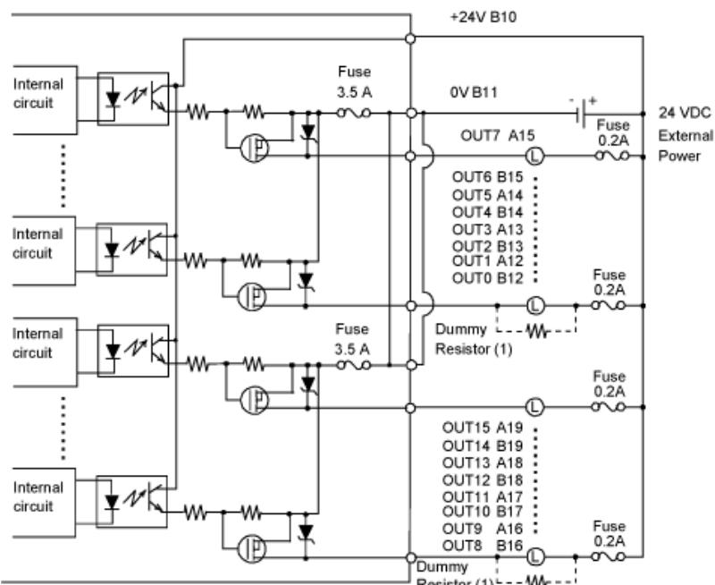
(1) (Example) The output delay time (OFF to ON) is 1.5  $\mu$ s where the output current is 50 mA. Install an external dummy resistor to increase the amount of current when faster response is required when the load is light.
