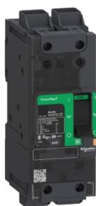
Circuit breaker, PowerPact B, 35A, 2 pole, 600Y/347VAC, 18kA, lugs, thermal magnetic, 80%
