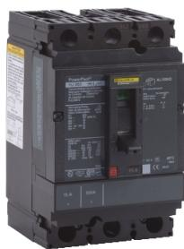
Circuit breaker, PowerPact H, 15A, 2 pole, 600VAC, 25kA, lugs, thermal magnetic, 80%
