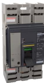
Automatic switch, PowerPacT P, 1200A, 3 pole, 600VAC, 25kA, busbar, magnetic, aux, shunt, motor op
