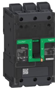
Circuit breaker, PowerPact B, 35A, 3 pole, 600Y/347VAC, 25kA, lugs, thermal magnetic, 80%
