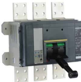
Circuit breaker, PowerPacT R, 2500A, 3 pole, 600VAC, 18kA, busbar, Micrologic 5.0, 100%
