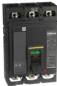
Circuit breaker, PowerPact M, 300A to 800A, 3 pole, 600VAC, 18kA, lugs, adjustable trip, 80%, shunt
