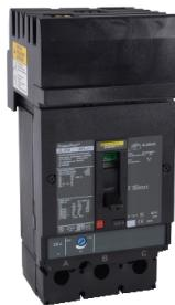
Circuit breaker, PowerPacT J, 150A, 3 pole, 600VAC, 50kA, I-Line, thermal magnetic, 80%, ABC
