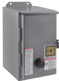
NEMA motor starter, Type S, nonreversing, Size 1, 27A, 10HP at 460VAC, 5kA SCCR, 3 phase, 3 pole, melting alloy, 208VAC coil, NEMA 12 [TAA]
