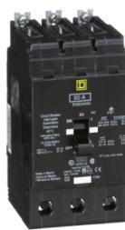
Mini circuit breaker, E-Frame, 50A, 3 pole, 480Y/277VAC, 65kA max, bolt on [TAA]
