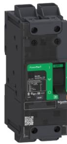
Circuit breaker, PowerPact B, 50A, 2 pole, 600Y/347VAC, 25kA, lugs, thermal magnetic, 80%
