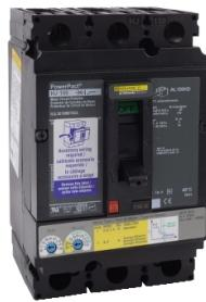
Motor circuit protector, PowerPact H, 150A, 3 pole, 600VAC, 25kA, lugs, thermal magnetic, 80%, shunt
