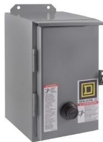
NEMA Motor Starter, Type S, nonreversing, Size 1, 27A, 10 HP at 460 VAC, 5 kA SCCR, 3 phase, 3 pole, melting alloy, 480 VAC coil, NEMA 12 [TAA]
