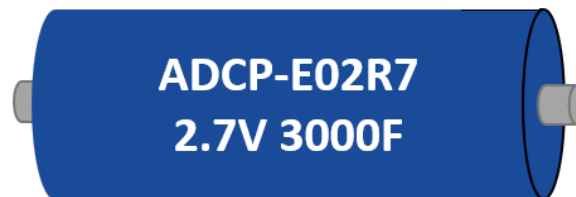
Example of the Markings of a 3000F 2.7V capacitor
