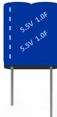
Example of the Marking of a 5.5V 1.0F Supercapacitor
