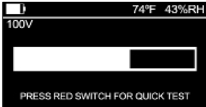
Figure 12. Electrification period timer
