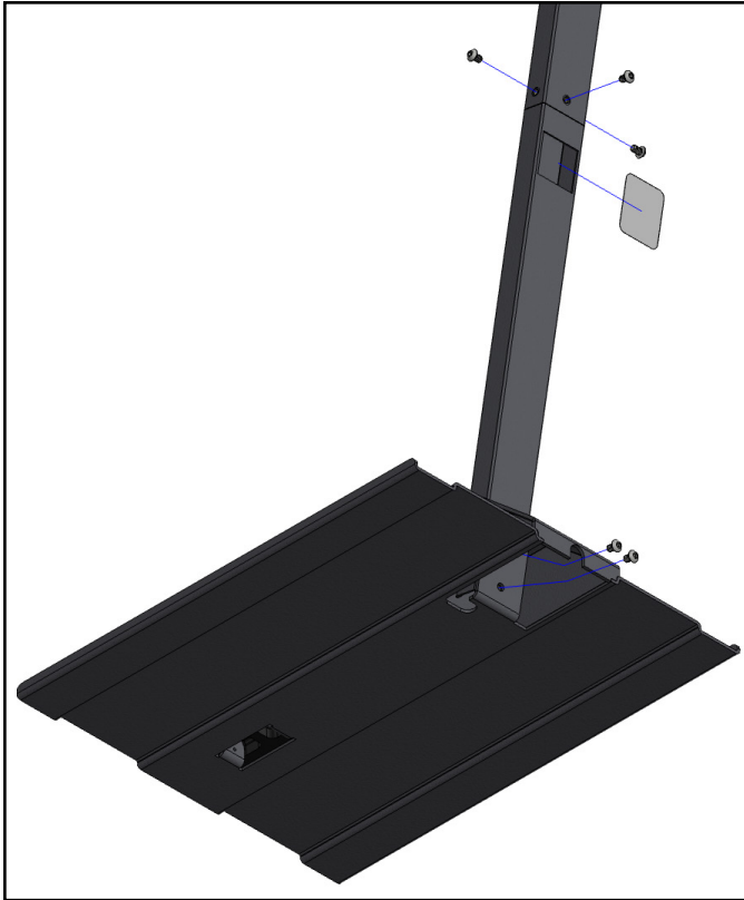
Figure 5. Assembling the pedestal and base plate using the 5 socket head screws
