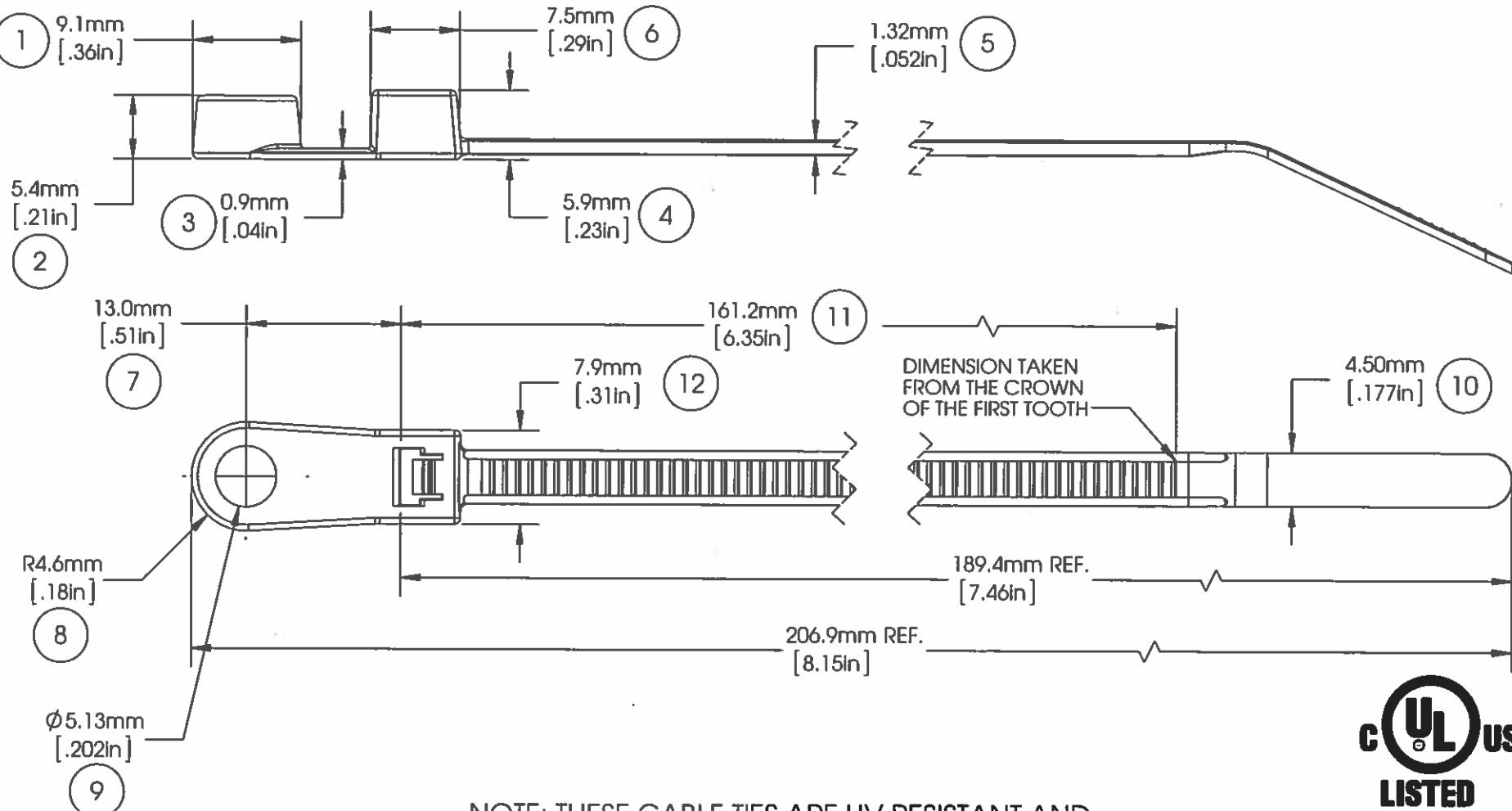
NOTE: THESE CABLE TIES ARE UV RESISTANT AND HAVE A FLAMMABILITY RATING OF V-2
