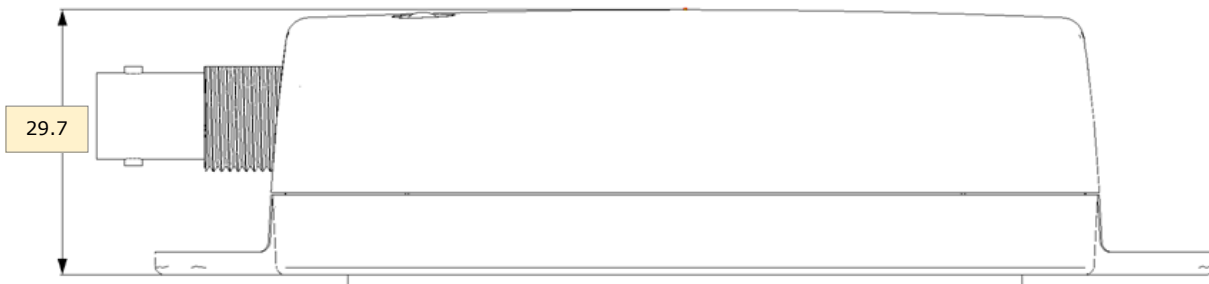
Figure 7 - Modbus ORP Sensor Adapter Dimension – Side View
