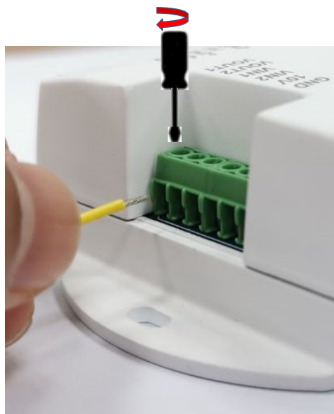
Figure 6 - Clamping wire with screwdriver in Clock-wise Direction
