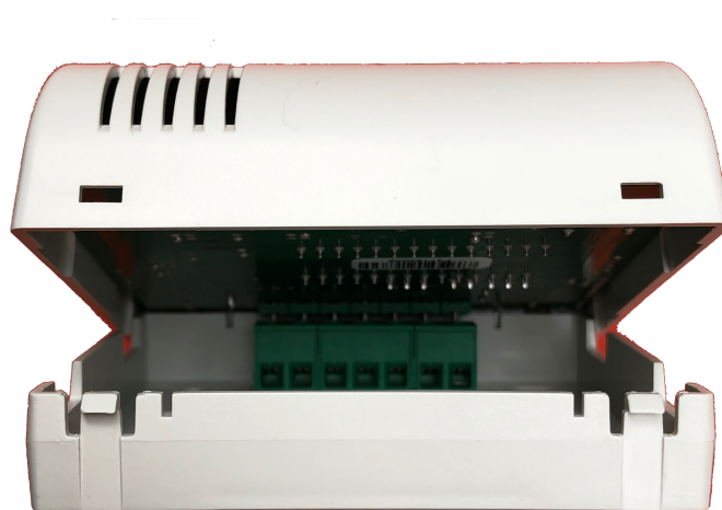
THE PCB HOLDERS OF THE FRONT COVER
