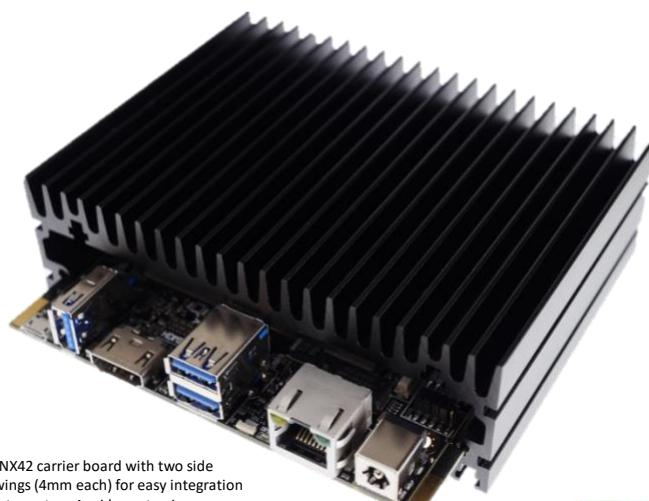
JNX42 carrier board with two side wings (4mm each) for easy integration into custom Auvidea extrusion
