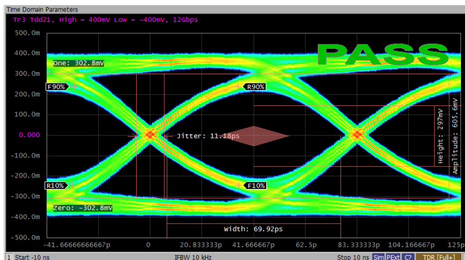
Figure 4. Data Rate 12Gb/s HDMI2.1 Eye Diagram without SY205227DVD
