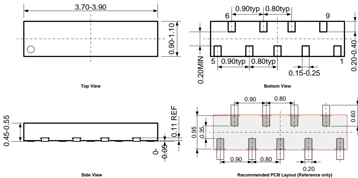
**Note:** All dimensions are in millimeters and exclude mold flash and metal burr.
