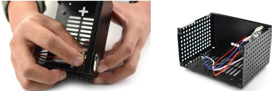
2. Next, install the reset switch to the corresponding holes, shown as below:
