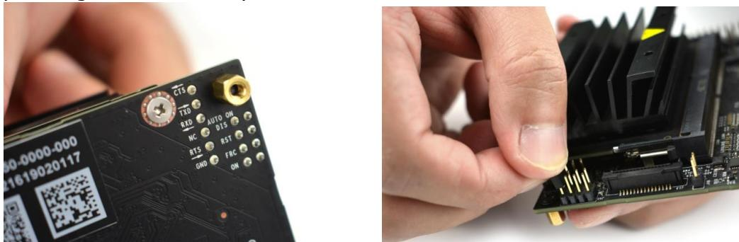
Plug the **RED** wire and the **Black** wire that control the power to pin "ON" in J40, and plug the **Blue** wire to "3.3V" and the **White** wire to "GND" in J41.
