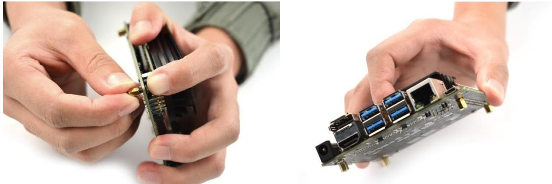
4. Plug the short-circuit cap to the position marked with "AUTO ON" to ban from powering ON automatically.
