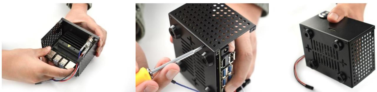
6. Finally, close the case cover, fix it with 4 screws. And the case installation is accompanied.
