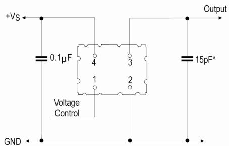
\* Inclusive of probe and jig capacitance
