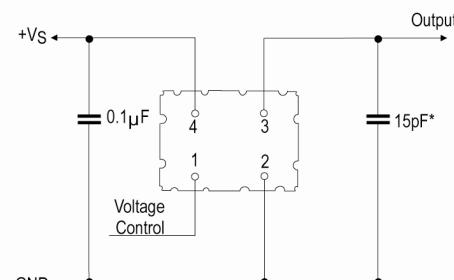
\* Inclusive of probe and jig capacitance
