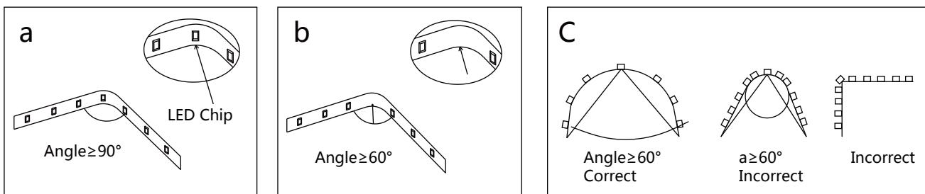
a: use an angle greater or equal to 90 degrees when there is an LED chip on the corner while placing the strip in a concave position (Angle $\geq$ 90degree)
