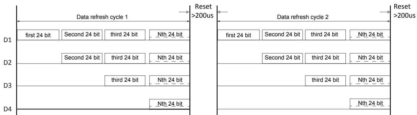
Note: Where D1 is the data sent by the MCU, D2, D3 and D4 are the data automatically shaped and forwarded by the cascade circuit.
