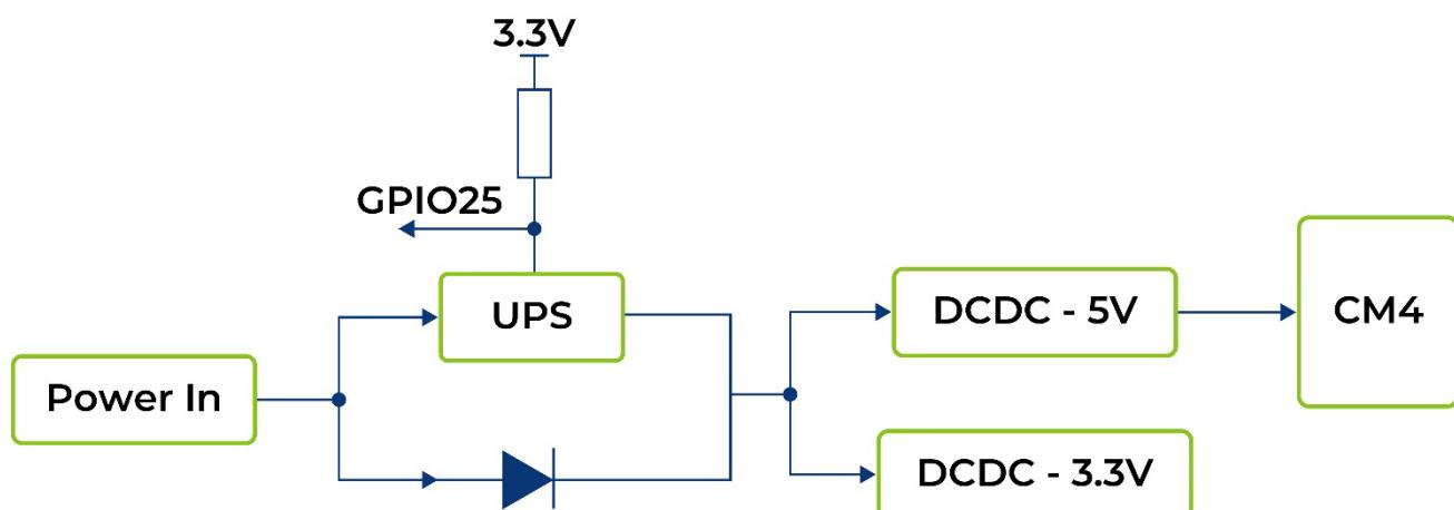
The UPS is 7F, which operates in series. The UPS module is positioned between the DC5V and CM4 components, with a GPIO signal utilized to alert the CPU in the event of a power loss from the 5V supply. Upon receiving this signal, the CPU executes an urgent script before the super capacitor's energy is depleted, initiating a "\$ shutdown" command.
