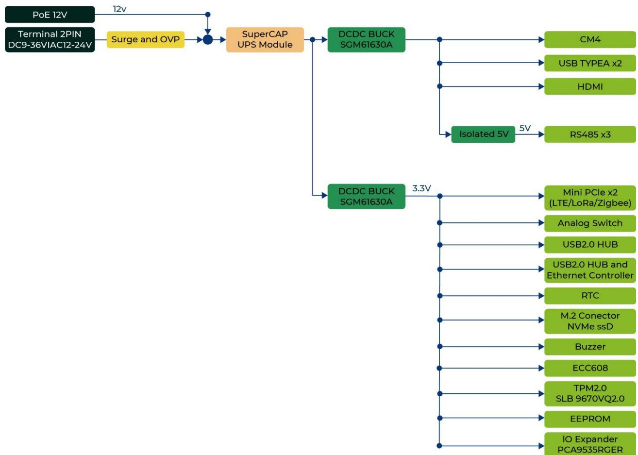
The reComputer R1000 supports three power supply options: AC, DC terminal and PoE port. By default, the reComputer R1000 is powered through the AC/DC terminal (Official regional power adapter SKU:110061505/110061506), while the PoE power supply(PoE module, SKU:110991925) is optional. This provides flexibility in power supply selection and allows for easy integration with various power sources.
