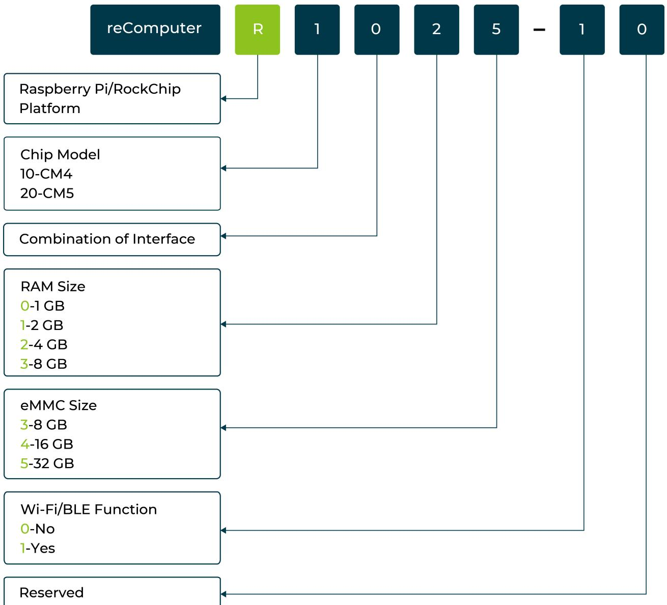
For example, the naming of 4GB RAM and 32GB eMMC CM4 module with Wi-Fi and BLE function tailored for smart building is reComputer R1025-10.
