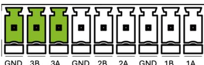
The reComputer R1000 is equipped with 3 sets of RS485 interface using 3-pin connector, which is isolated for both signal and power to ensure safe and reliable operation in industrial and automation applications. The RS485A and RS485B signals are isolated using capacitive isolation, which provides excellent EMI immunity and meets the high-speed communication requirements of the RS485 interface.
