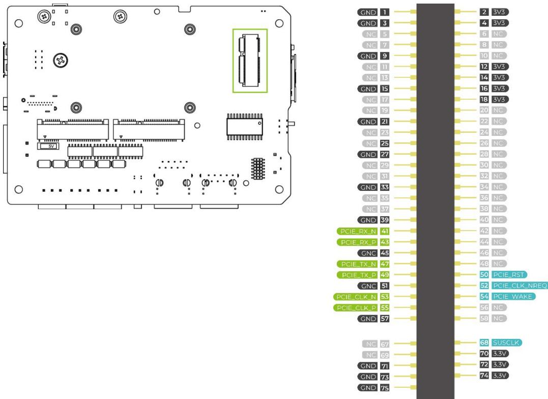
The SSD slot on the reComputer R1000 is designed to accommodate NVMe M.2 2280 SSDs for 128GB, 256GB, 512GB and 1TB in capacity. This slot allows for high-speed storage expansion, enabling users to enhance the performance and capacity of their system.
