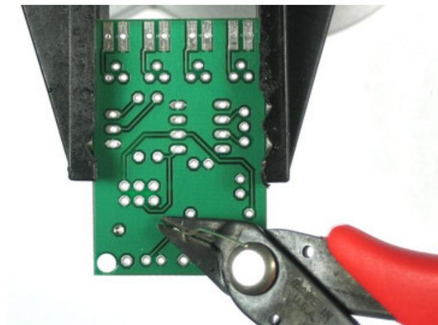
Use the diagonal cutters to clip off the resistor legs so that only the solder points remain.
