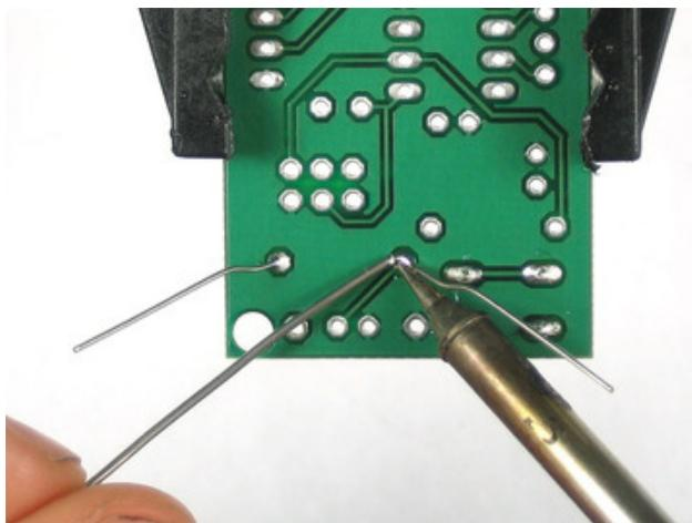
Solder each leg of the resistor.
