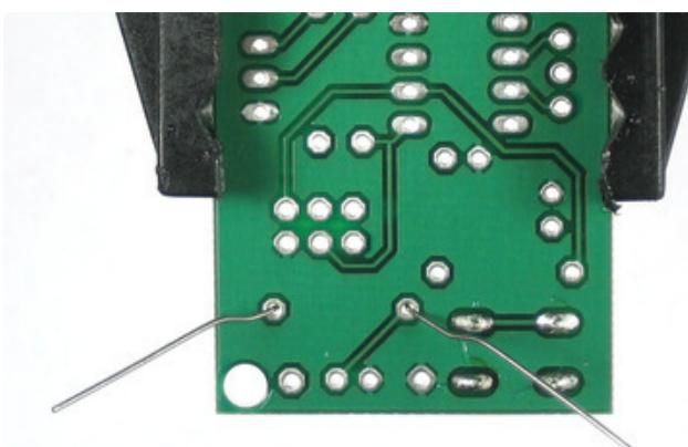
Next is the 1.0 kilo ohm resistor **R5**. This is the brown-black-red striped part. This resistor sets the brightness of the little indicator LED. Resistors are symmetric, so it can go in either way.
