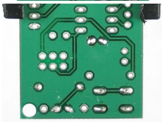
Solder and clip the ceramic capacitor part.
