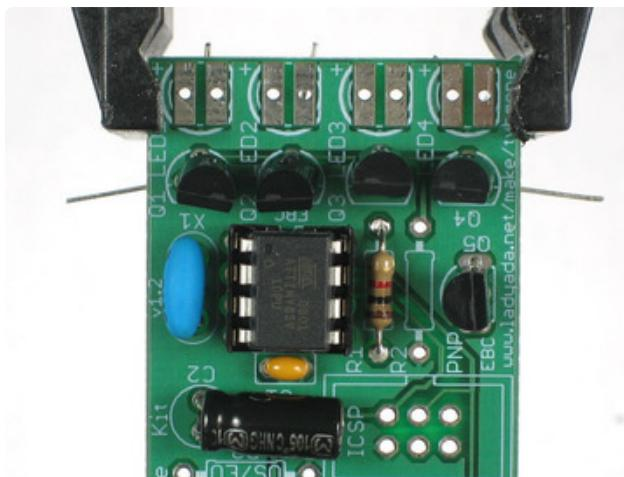
Next are the four NPN (2N2222) transistors **Q1** **Q2** **Q3** and **Q4**. These are the devices that turn on and off the high power IR LEDs. The microcontroller doesn't have the capability to provide a lot of power directly to the LEDs so these transistors assist it.
