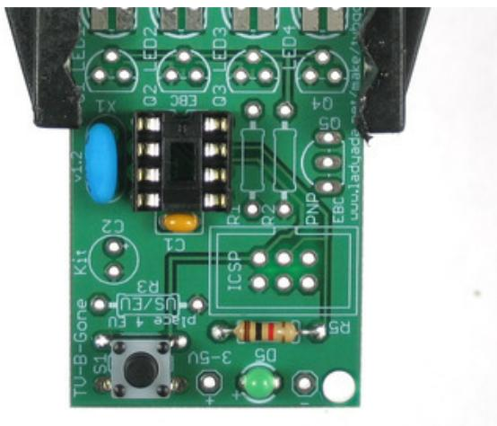
The socket is for protecting the chip and making it easy to insert and remove.
