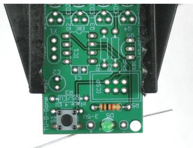
Insert the LED into the correct location, and bend the leads out to keep it from falling out when you turn the PCB over.
