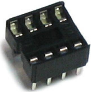
A black plastic DIP-8 package, which is an 8-pin socket used for prototyping or reprogramming the microcontroller.                                                                                                 | IC1' | 8-pin socket                                                     | Generic                                                                             |
