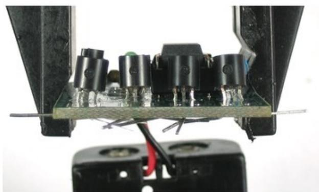
Transistors have three pins. Bend the middle pin back a little and insert it so that the rounded and flattened sides match up with the picture silkscreened onto the circuit board, as shown. The transistor won't be able to sit flat against the circuit board, so just make it poke up a few millimeters.
