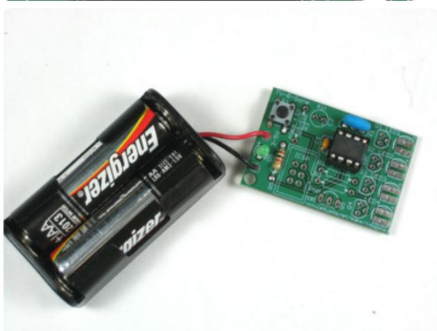
The microcontroller is the device that stores all the codes and turns the LEDs on and off according to a program.
