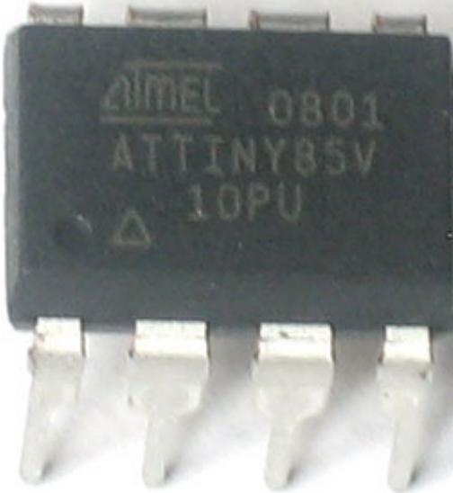
A black plastic DIP-8 package of an ATtiny85 microcontroller. The package is marked with the text 'ATMEL 0801 ATTINY85V 10PU' and a small triangle symbol. The package is labeled 'IC1' in the bottom right corner. | IC1  | Microcontroller<br>(preprogrammed<br>when purchased<br>in a kit) | ATTINY85V-10-<br>PU<br><br>(unprogrammed<br>when not<br>purchased from<br>Adafruit) |
