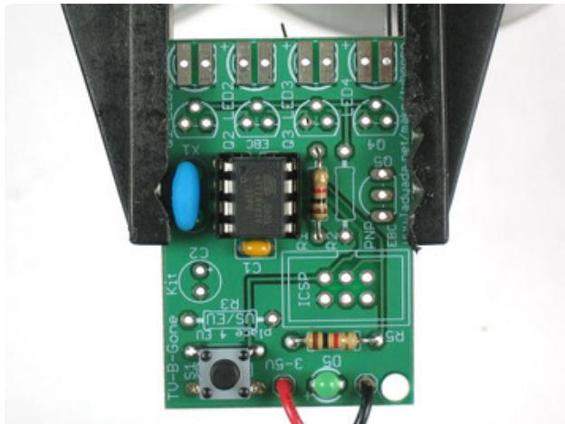
Next place the 1.0K ohm resistors, **R1**. This is the base resistor for the PNP transistor.
