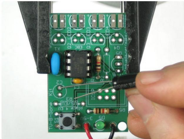
Next is the 220uF electrolytic capacitor. It is polarized so make sure it goes in the right way. The long lead is positive, and goes into the hole marked with a +, on the right in this photo.
