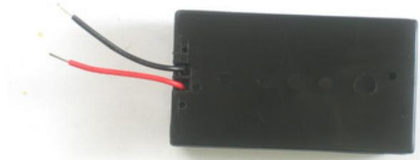
Strip the ends of the wire off so that there's a short section without insulation.
