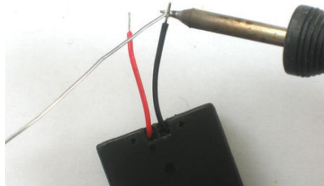
Use your soldering iron to 'tin' the wire, melting solder into it to keep the wire from fraying.
