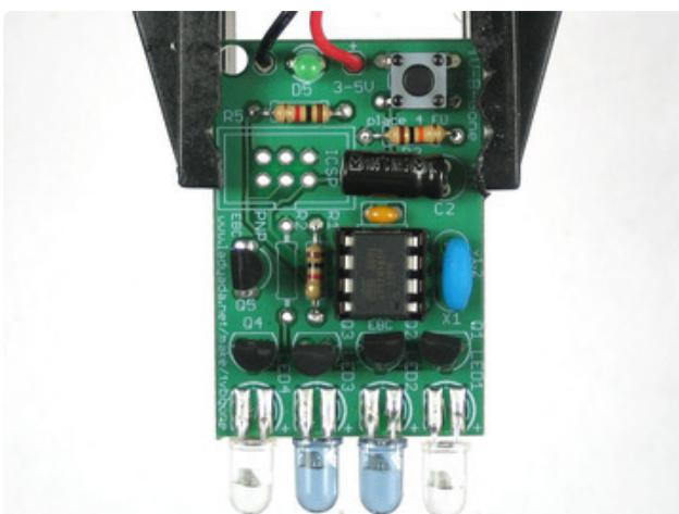
If you're in the EU, UK, Australia, place the remaining 10K resistor into **R3**. This will tell the microcontroller to use the EU database.
