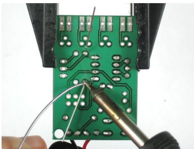
Solder and clip the resistor.
