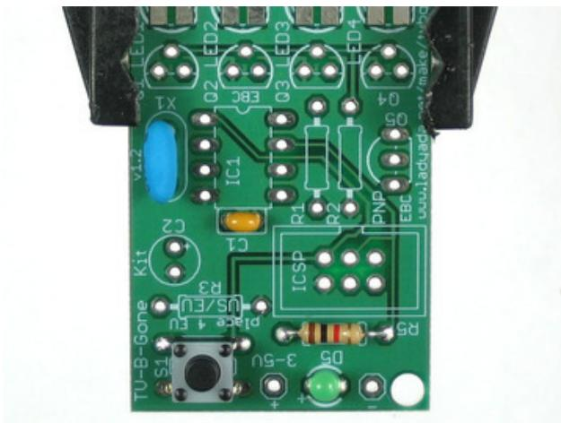
Next, place 2 components. The ceramic oscillator and the 8-pin socket. The oscillator has 3 pins and is symmetrical. The oscillator is the timeclock for the microcontroller, making sure that it is performing its functions at the correct speed.
