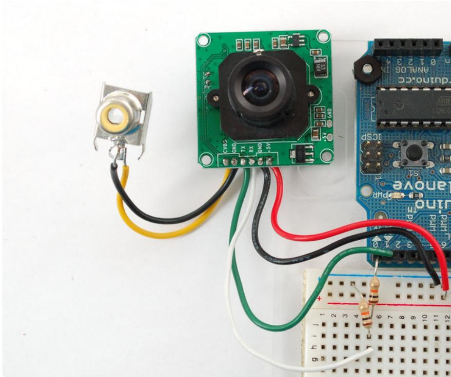
For the weatherproof camera, the white and green wires are swapped on some cameras! So please flip the white and green wires indicated if using the metal camera. Red should still be connected to +5 and Black to Ground
